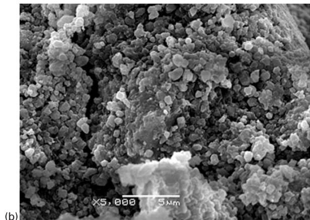
a dependence of compressive strength on processing pressure and temperature; b SEM of fracture surface after 15 min of hot pressing
